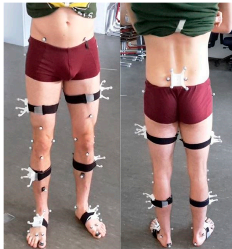
Figure 1. Instrumentation of one exemplary subject. Marker set and rigid marker clusters.
